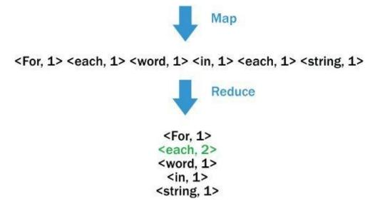
**Figure 10.1** Example of how MapReduce works
