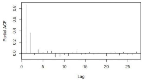
Figure 8.4 Partial autocorrelation function (PACF) plot
