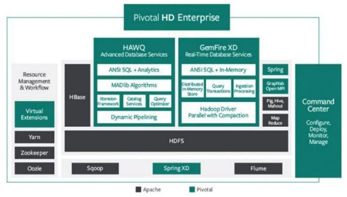
Figure 10.7 Components of Pivotal HD Enterprise
